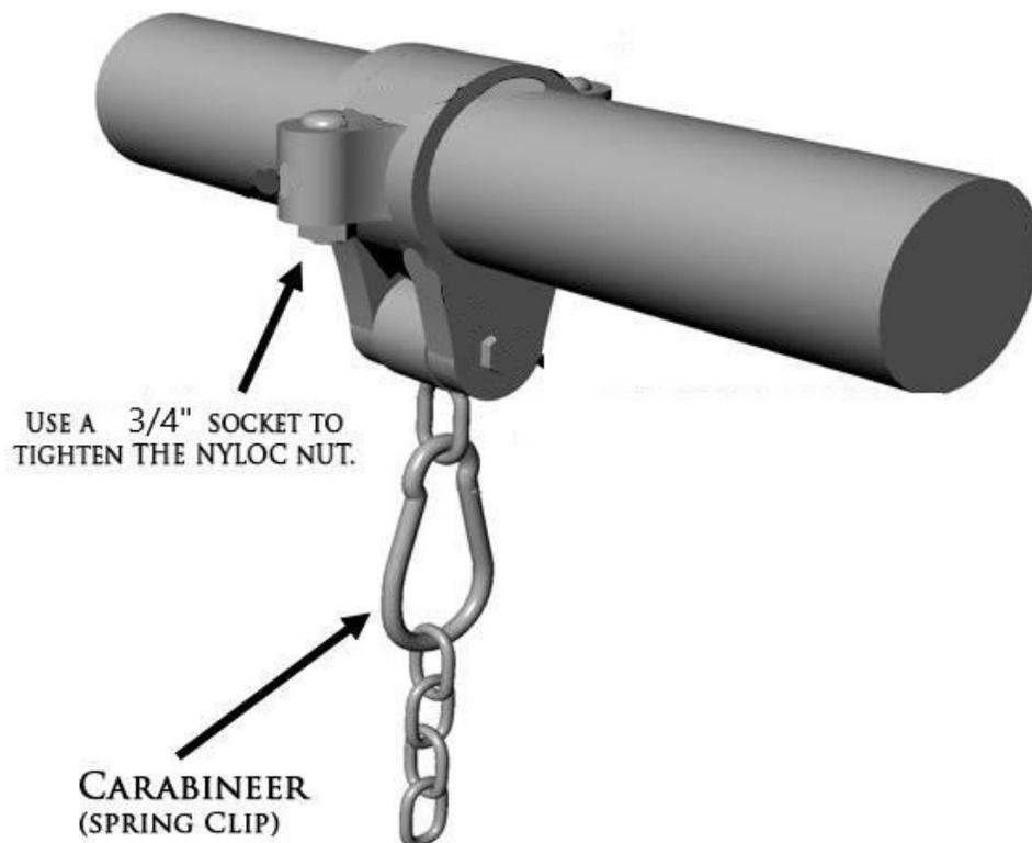
**1. Loosen and remove the two nyloc jam nuts. 2. Reassemble on to swing top rail. Tighten securely so that the hanger is firmly attached in place and cannot slide or swivel along top rail. 3. Attach carabineer with chain through the ring.**
