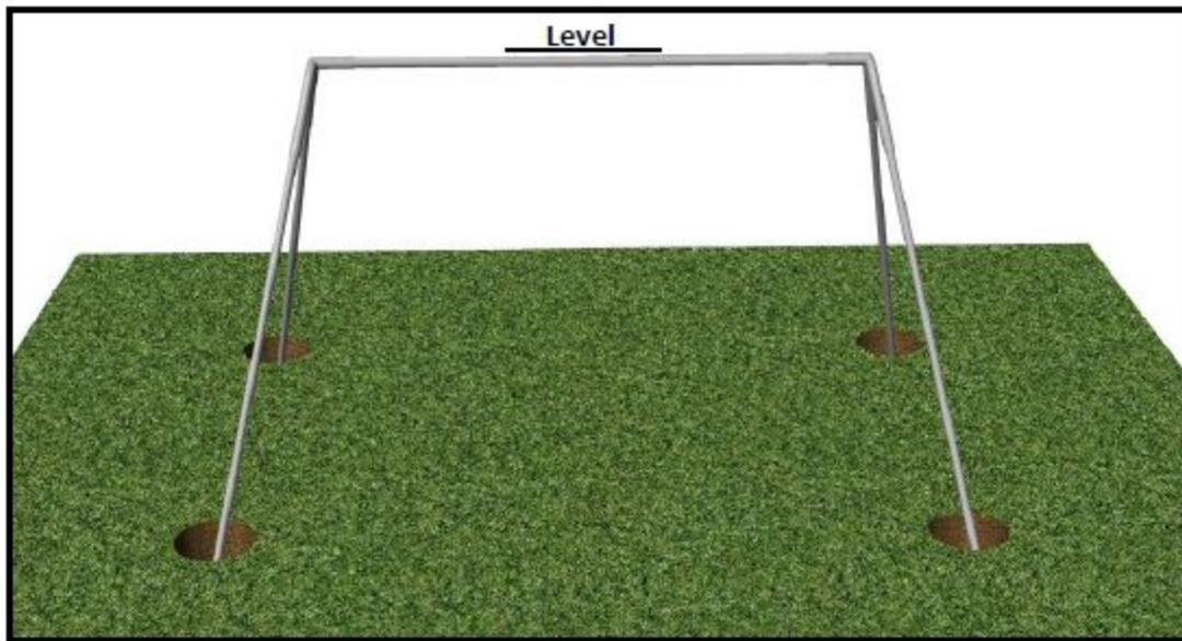
When you are satisfied that the structure is level, mix and pour the concrete according to the package directions. You will use approximately one and a half to two 80 lb. bags in each leg hole.
