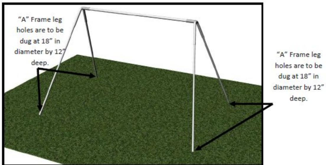
Place the set into the holes. Align the legs.
