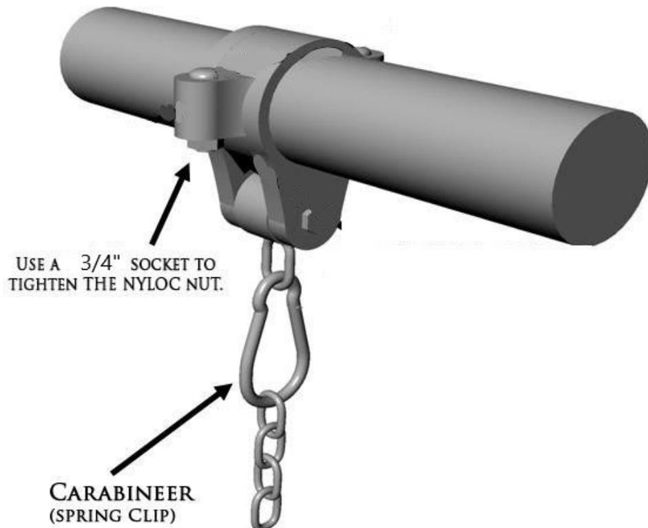
**1. Loosen and remove the two nylock jam nuts. 2. Reassemble on to swing top rail. Tighten securely so that the hanger is firmly attached in place and cannot slide or swivel along top rail. 3. Attach carabiner with chain through the ring.**
