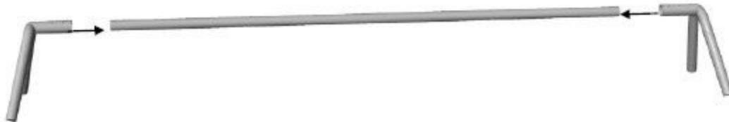
**Step 1:** Slide the ends of the 10' Top Rail as far as it will go into the Sleeves of the Triple Ends.
