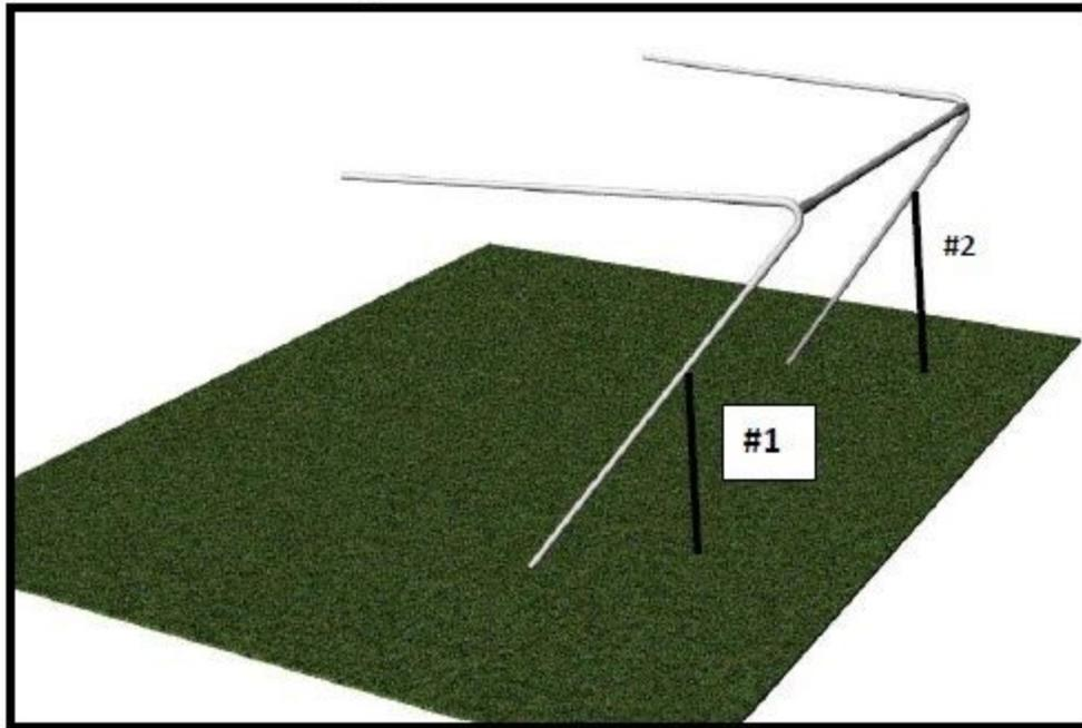
Mark holes around a-frame leg, move set to the side of markings and dig holes.
