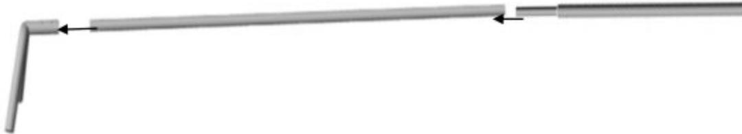
**Step 1:** Slide the undrilled end of the longer Top Rail as far as it will go into the Sleeve of the Triple End
