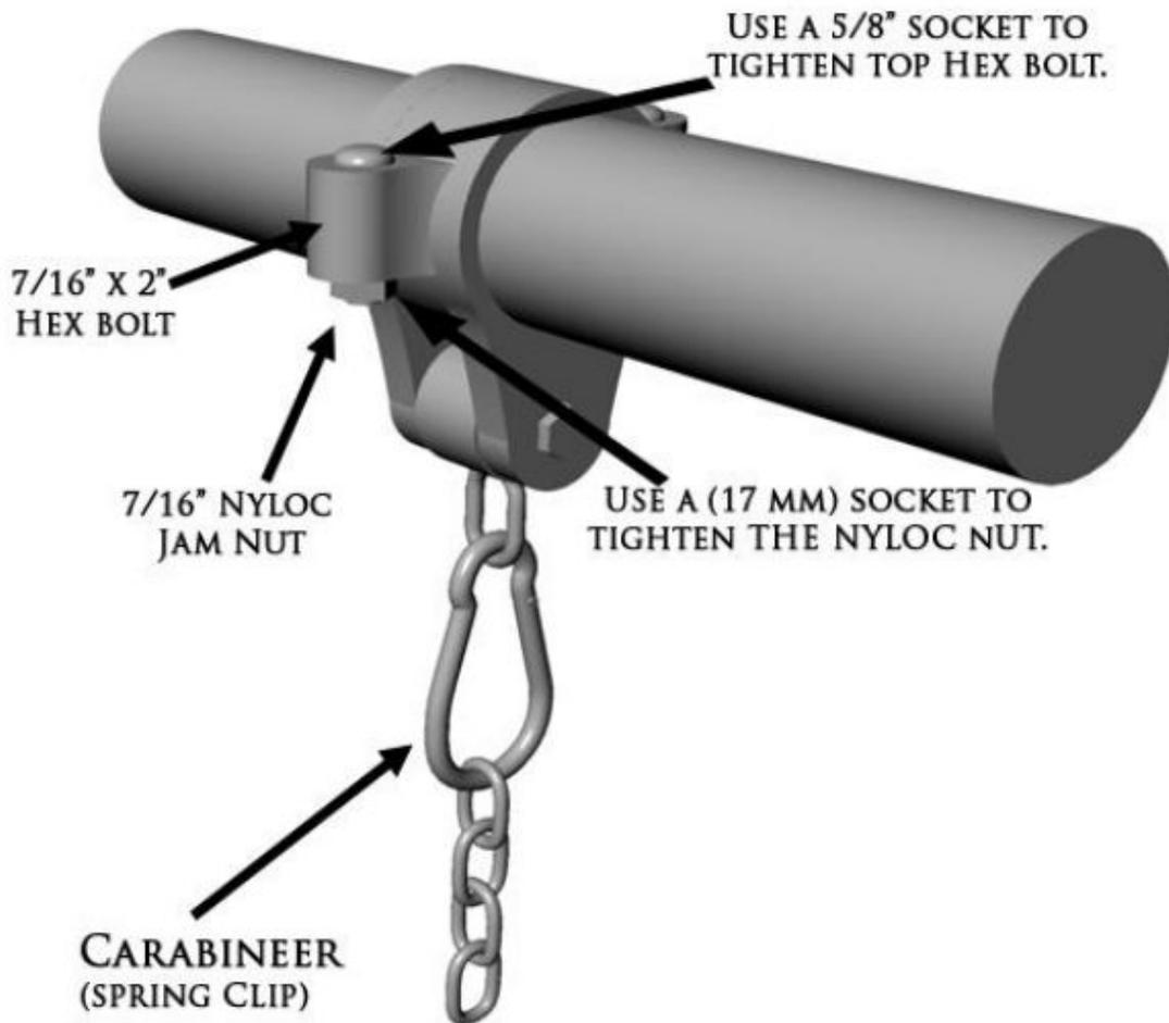
1. Loosen and remove the two nyloc jam nuts.
